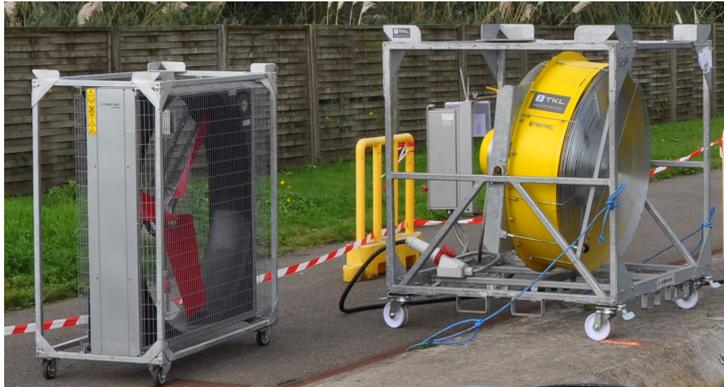
Fig. 3.2 – View of the two fans, TROTEC TTW 45000 : 2 m/s (left) and TROTEC TTW 100000 : 5 m/s and 8 m/s (right)
