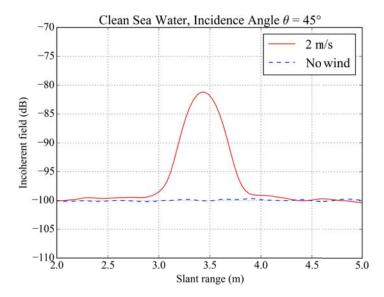
**Figure 7.** Incoherent field of the clean seawater surface with an incidence angle of  $45^{\circ}$  in VV polarization at  $10.5\,\text{GHz}$ . Two configurations are observed: a seawater state with a wind speed of  $2\,\text{m/s}$  (red line) and a flat seawater surface (blue dashed line).
