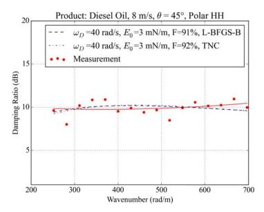
Figure 16. Damping ratios calculated for diesel oil spill by considering a wind speed of  $8 \,\mathrm{m/s}$  in HH polarization for an incidence angle of  $45^\circ$ . The data points (red dots) are fitted by a third-degree polynomial (red line). The dashed lines are the damping ratios obtained from the minimization process (black dashed line: L-BFGS-B method, blue dotted line: TNC method).
