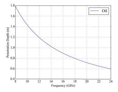
Figure 12. Oil penetration depth.
