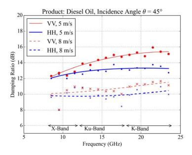
**Figure 8.** Damping ratios from the diesel oil spill acquired at two different wind speeds (5 and  $8 \,\mathrm{m/s}$ ) in VV (red) and HH (blue) polarizations with an incidence angle of  $45^{\circ}$ . The lines are third-degree-polynomial fits on the acquired data points (dots and crosses).
