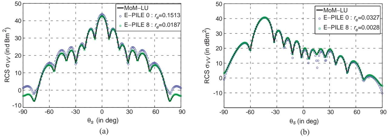
**Figure 6.** Convergence of E-PILE versus its order, for the case of two parallel plates,  $S_1 = 2\lambda_0 \times 2\lambda_0$ ,  $S_2 = 6\lambda_0 \times 6\lambda_0$ ,  $D = 5\lambda_0$ : (a)  $\theta_i = 0^\circ$ , (b)  $\theta_i = 45^\circ$ .
