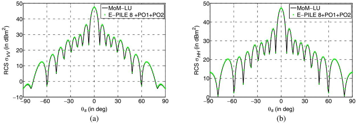
**Figure 10.** Comparison of the radar cross-section of two parallel plates computed from the hybrid method (EPILE 8+PO1+PO2) with that obtained from the reference method (MoM-LU) versus the scattering angle. The parameters are  $S_1 = 1\lambda_0 \times 1\lambda_0$ ,  $S_2 = 8\lambda_0 \times 8\lambda_0$ ,  $D = 5\lambda_0$ ,  $\theta_i = 0^\circ$ : (a) vertical polarization, (b) horizontal polarization.
