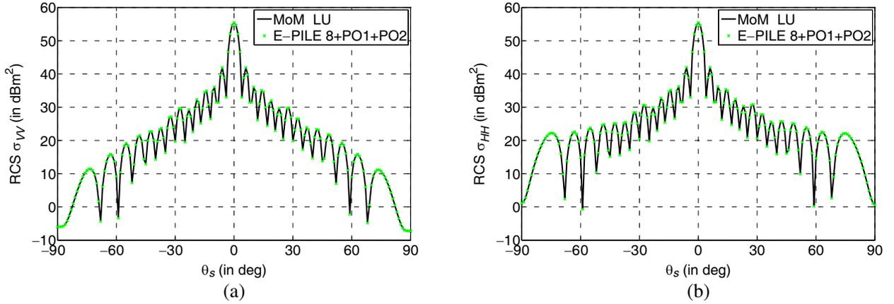
**Figure 13.** Comparison of the radar cross-section of two parallel plates computed from the hybrid method (EPILE 8+PO1+PO2) with that obtained from the reference method (MoM-LU) versus the scattering angle. The parameters are  $S_1 = 2\lambda_0 \times 2\lambda_0$ ,  $S_2 = 14\lambda_0 \times 14\lambda_0$ ,  $D = 5\lambda_0$ ,  $\theta_i = 0^\circ$ : (a) vertical polarization, (b) horizontal polarization.
