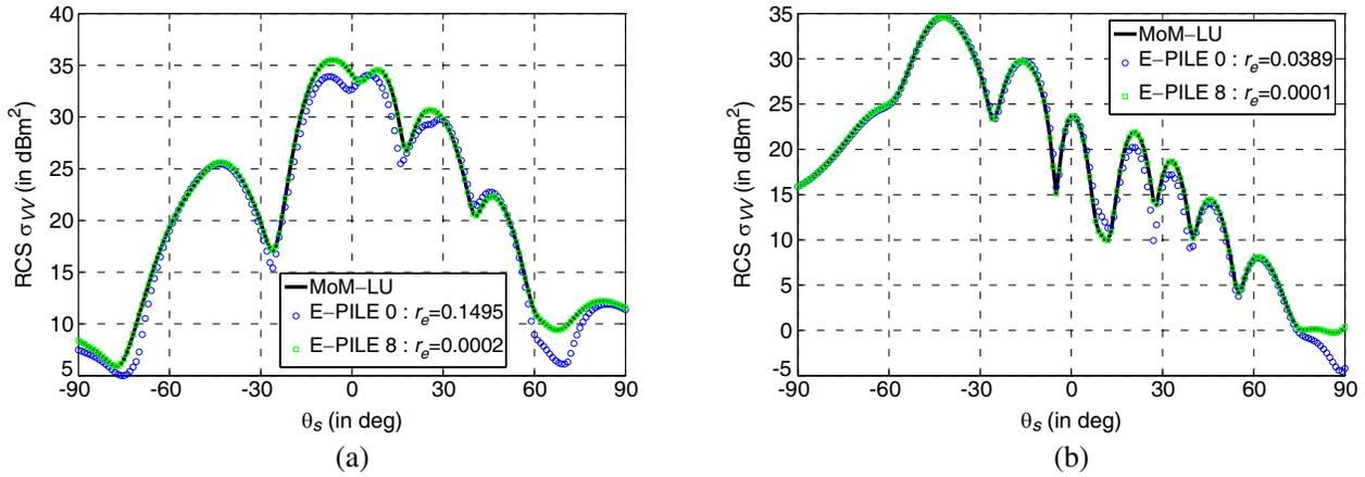
Figure 8. Convergence of E-PILE versus its order, for the case of a plate above a rough surface,  $S_1 = 2\lambda_0 \times 2\lambda_0$ ,  $S_2 = 6\lambda_0 \times 6\lambda_0$ ,  $D = 5\lambda_0$ ,  $\sigma_z = 0.2\lambda_0$ ,  $L_{cx} = L_{cy} = 1\lambda_0$ : (a)  $\theta_i = 0^\circ$ , (b)  $\theta_i = 45^\circ$ .
