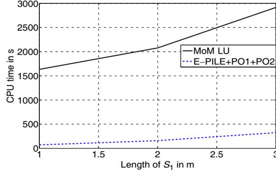
**Figure 15.** Comparison of computing time of the hybrid and rigorous method versus the length of  $S_1$  for the case of two parallel plates  $S_1$  above  $S_2$ .
