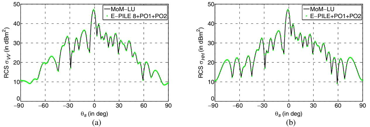
**Figure 14.** Comparison of the radar cross-section of a plate above a rough surface computed from the hybrid method (EPILE 8+PO1+PO2) with that obtained from the reference method (MoM-LU) versus the scattering angle. The parameters are  $S_1 = 2\lambda_0 \times 2\lambda_0$ ,  $S_2 = 14\lambda_0 \times 14\lambda_0$ ,  $D = 5\lambda_0$ ,  $\sigma_z = 0.2\lambda_0$ ,  $L_{cx} = L_{cy} = 1\lambda_0$ ,  $\theta_i = 0^\circ$ : (a) vertical polarization, (b) horizontal polarization.
