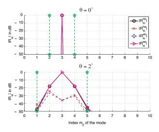
**Figure 7.** Moduli of the elements of the reflection matrix  $\bar{\mathcal{R}}_{is}$  given by Eq. (31) versus the index of the mode  $m_2$  and the tilt angle  $\theta_{12} = \{0, 2\}^{\circ}$ .  $a_1 = b_1 = 8\lambda_0$ , n = 2, and  $m_1 = 3$ .
