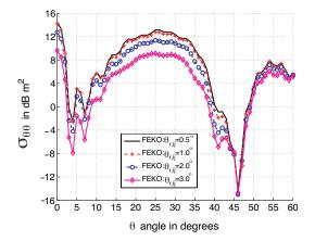
**Figure 14.** Monostatic RCS  $\sigma_{\theta\theta}$  in dB m<sup>2</sup> versus  $\theta$  and  $\theta_{r,ij} = \{0.5, 1, 2, 3\}^{\circ}$ .  $a_1 = b_1 = 8\lambda_0$ ,  $L_1 = 5\lambda_0$ ,  $L_1 = L_2 = L_3 = \lambda_0$ , and  $\phi = 0$ .
