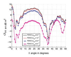
**Figure 8.** Monostatic RCS  $\sigma_{\theta\theta}$  in dB m<sup>2</sup> versus  $\theta$  and  $\theta_{12} = \{0, 1, 2, 5\}^{\circ}$ .  $a_1 = b_1 = 8\lambda_0, L_1 = 5\lambda_0, L_2 = 4\lambda_0$ , and  $\phi = 0$ .
