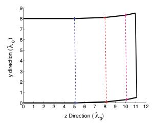
Figure 2. Cavity of rectangular and *uniform* cross section along the  $\hat{\mathbf{z}}$  direction, and modeled as a succession of 3 bends.  $b_1 = 8\lambda_0$  ( $a_1 = 8\lambda_0$ ),  $L_1 = 5\lambda_0$ ,  $L_2 = 3\lambda_0$ ,  $L_3 = 2\lambda_0$ ,  $L_4 = 1\lambda_0$ ,  $\theta_{12} = 2^\circ$ ,  $\theta_{23} = 4^\circ$  et  $\theta_{34} = 6^\circ$  ( $\theta_{r,12} = \theta_{r,23} = \theta_{r,34} = 2^\circ$ ).
