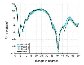
**Figure 3.** Monostatic RCS  $\sigma_{\theta\theta}$  in dB m<sup>2</sup> versus  $\theta$  and  $p_1 = \{1, 2, 3\}$ .  $a_1 = b_1 = 8\lambda_0, L_1 = 9\lambda_0$ , and  $\phi = 0$ .
