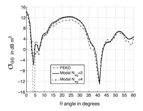
**Figure 18.** Same as in Fig. 10  $(N_{\text{wg}} = 2 \text{ with } \theta_{12} = 2^{\circ} \text{ and } L_2 = 4\lambda_0)$  but the results obtained from  $N_{\text{wg}} = 4$   $(\theta_{12} = \theta_{23} = \theta_{34} = 1^{\circ} \text{ and } L_2 = L_3 = L_4 = 1.3335\lambda_0)$  are added.
